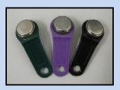
iButtons and iButton readers are not magnetic but are fully electronic. iButtons are very resistant to water and shock. iButtons are also available in various types, and when desired are installed in various colored plastic keyring tags. The color has no particular meaning. Only DS1990 iButtons and user keypad codes are used as 'User keys' when programming E4 / E5 locks via the keypad. (DS1977 iButtons are used to program locks only when using PC computer software to program locks.)
