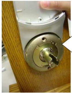
Step 8: Install Inside Rose Insert: (Avoid to catch the wire when insert the top mounting screw.)
