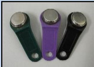
iButtons and iButton readers are not magnetic but are fully electronic. iButtons are very resistant to water and shock. iButtons are also available in various types, and when desired are installed in various colored plastic keyring tags. The color has no particular meaning. Only DS1990 iButtons and user keypad codes are used as 'User keys' when programming E4 / E5 locks via the keypad. (DS1977 iButtons are used to program locks only when using PC computer software to program locks.)
