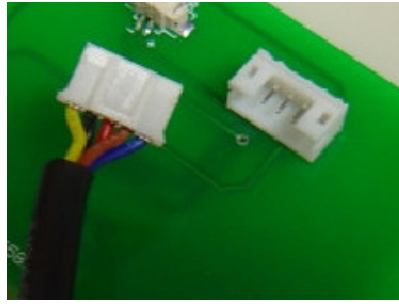
Step 5: Connect to battery case before hook the battery case in place
